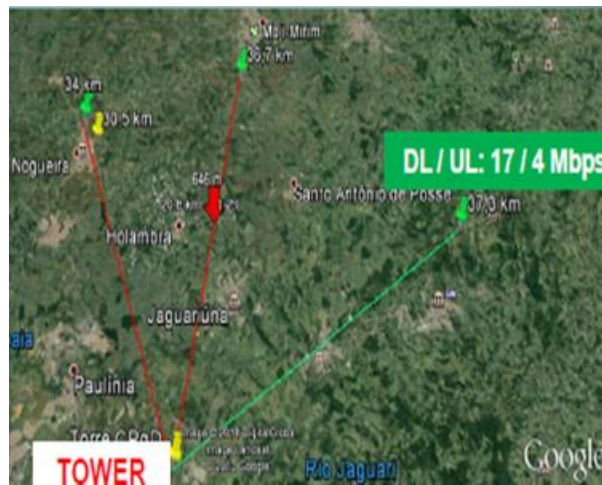
Figure 272 - Example one of life network measurement of LTE450 performance
